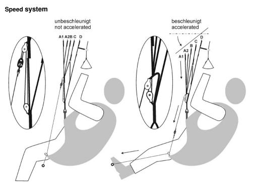
Fig. 5: How the Arcus 7 speed system works
