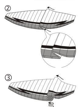
Vary slightly the final step of packing up ④, so that it is not always the middle cell which is bent. Use the neighbouring cells as well from time to time to increase the life of the fabric, particularly in the middle part.
