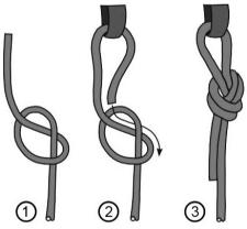
Fig. 2: Overhand knot
