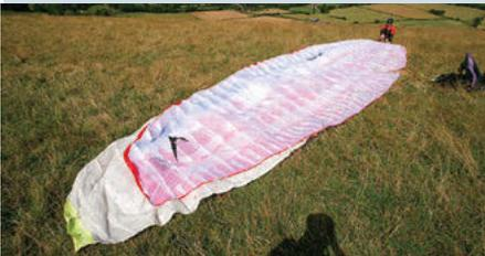
Incredibly, the Swing Discus has only a smidge less aspect ratio than the cutting edge comp wing of yesteryear. The Nexon only has 10cm less chord in the centre section and 40cm more span.
