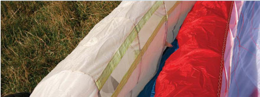
Fifteen years ago, performance relied on narrow aerofoil sections that were inherently prone to collapsing. Modern A-class wings gain the same performance through much more efficient profiles. Even though they're much fatter and chunkier to look at, they generate much better lift, less drag, and are inherently much more stable.
