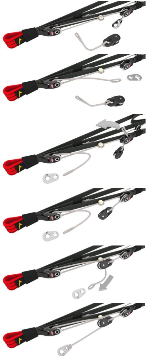
Fig. 10 Installing the speedlimiter
