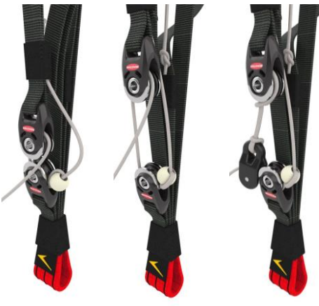
Fig. 9 MIURA RS riser at speed steps with and without speed limiter
