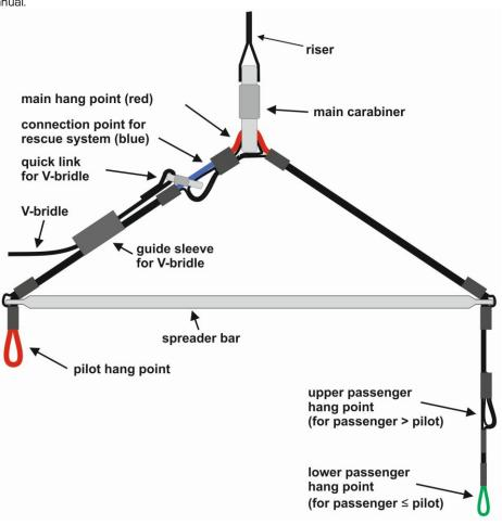
Fig. 8 Tandem spreader bar
