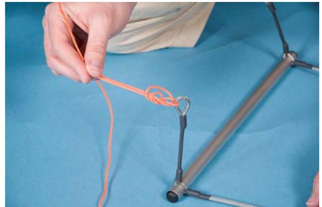
**Fig. 6-17: Knot fastening the speed bar**
