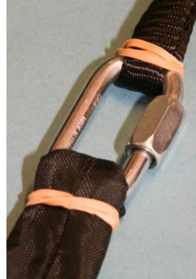
**Fig. 5-5: Screw link with rubber bands**
