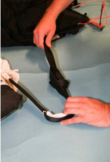
**Fig. 5-3: Tighten the loops where attached**
