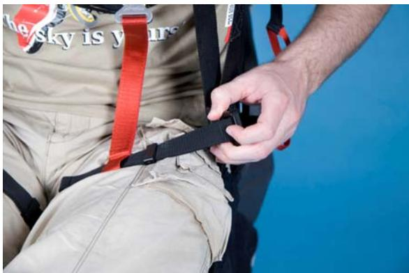
**Fig. 6-12: Lengthening the leg straps**
