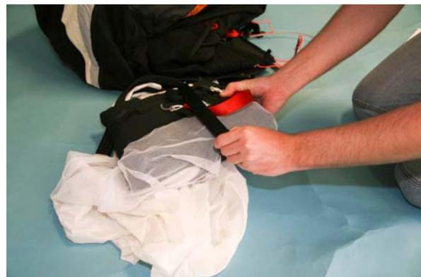
**Fig. 5-2: Feed the reserve through the loop of the bridle**
