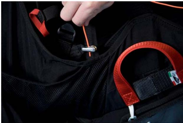
**Fig. 6-14: Speed bar line through pulley**
