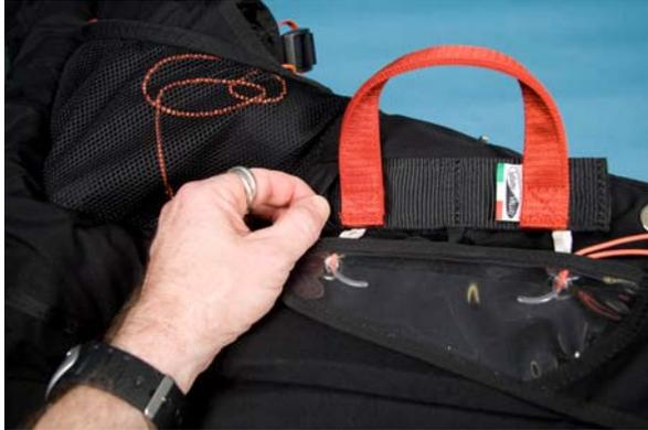
**Fig. 5-18: Put in the ends of the deployment handle**
