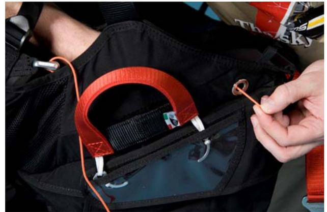
**Fig. 6-15: Speed bar line through eyelet**
