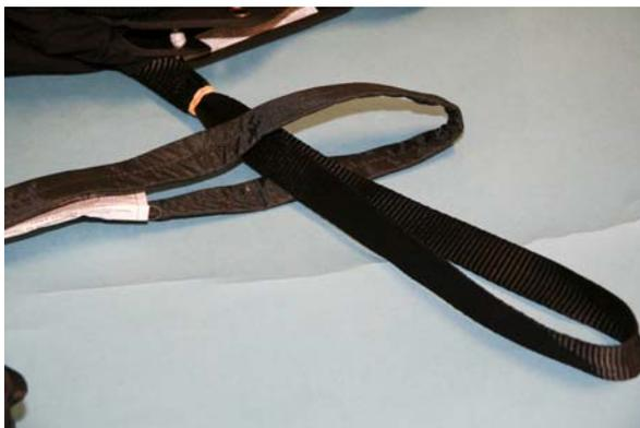
**Fig. 5-1: Put the bridle through the riser**
