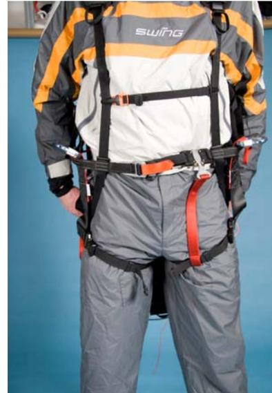
**Fig. 10-6: Do up the connecting strap**
