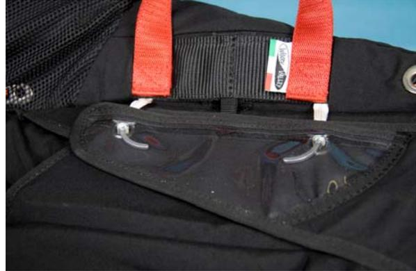
**Fig. 5-19: Outer container closed with pack cords removed**
