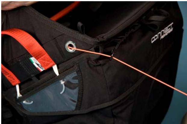
**Fig. 6-16: Speed bar line through eyelet, and plastic ring**
