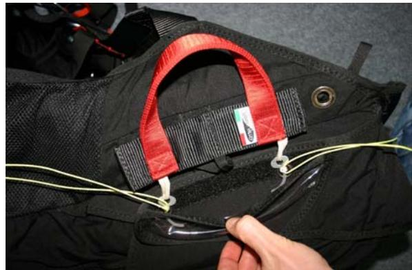
**Fig. 5-17: Release pin inserted**
