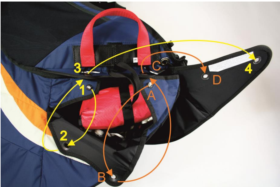
Fig. 6: Reserve in the reserve container, sequence for closure shown
