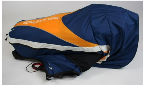
Fig. 27: Harness ready to fly (Airbag prepared)
