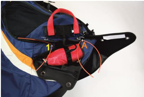
Fig. 7: Elastic closures with pack cord/tube
