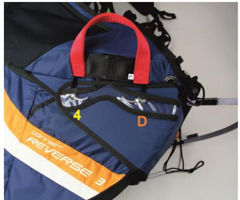
Fig. 5: Front flap secured with pins, deployment handle stowed away
