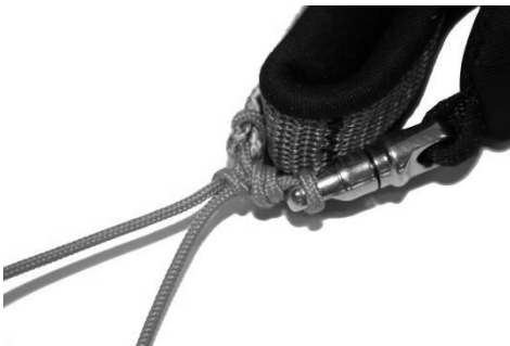
Fig. 8 Knot on the brake handle
