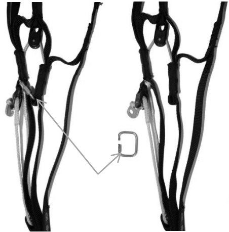
Fig. 13 MITO riser with and without speed limiter
