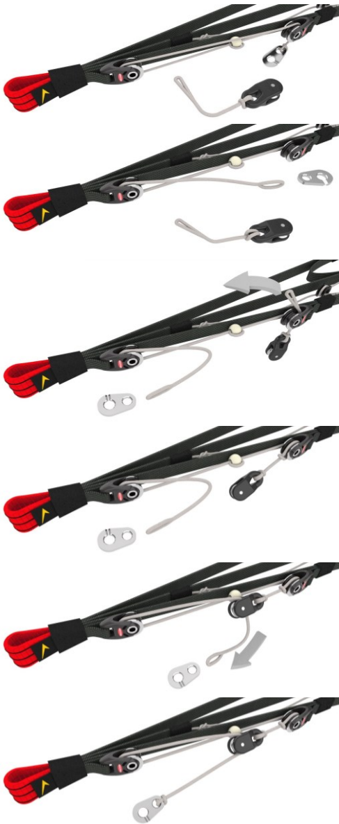
Fig. 9 Installing the speedlimiter
