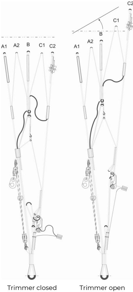
Fig. 14 How the trimmers work
